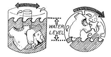
Conventional top-loading washers (left) use a large vertical drum. Most high-efficiency washers (right) utilize a horizontal-axis design; loading from the front, they tumble clothes through a much smaller pool of water. There are currently three high-efficiency washing machines on the residential market (Whirlpool, Staber and Fisher-Paykel) that are top-loading.
